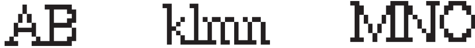
Figure 9.4: Glyphs extracted from text that uses proportional spacing, and where the characters are too close together to be easily separated. The fact that the characters are connected by black pixels leads to the problem of selecting a location at which to split them.
