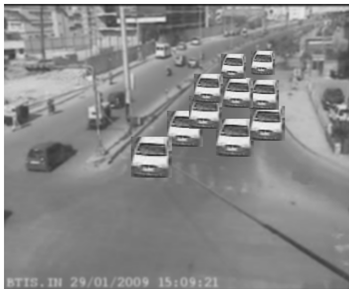
Figure 5. Synthetic traffic data with different number of vehicles. (a)1, (b)3, (c)5, (d)10, (e)13 and (f)17
